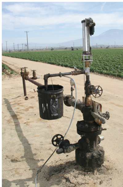
MK's Rhino MiniJack™ Pneumatic Piston Pump pumping oil at a U.S. field.
