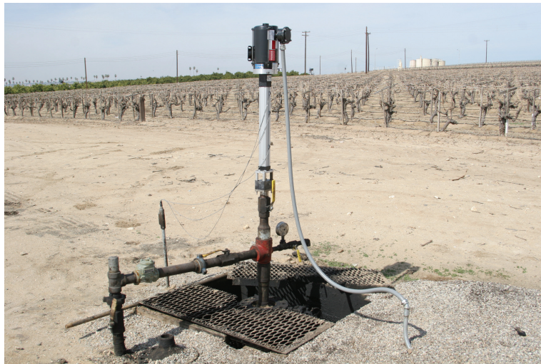
MK's Rhino MiniJack™ Electric Piston Pump recovering oil from a U.S. stripper well.
